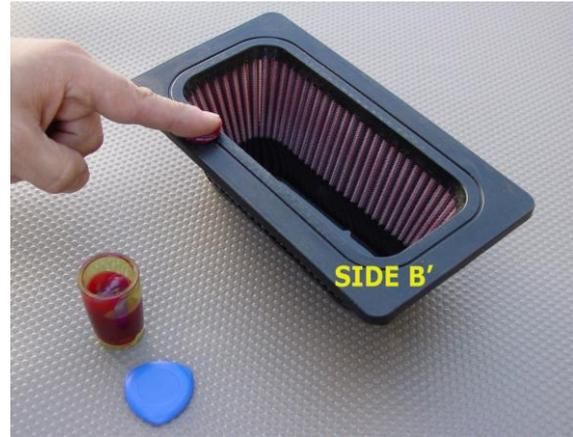
Push carefully the DNA filter all way down the air box,
